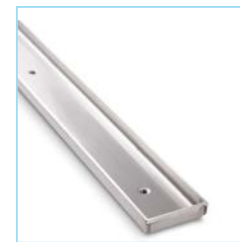
13 Exclusive tileable drain cover for Fundo Riolito: can be tiled with epoxy glue/adhesive or wedi Joint Sealant- used with 1/4 inch (6.4 mm) and 1/2 inch (12.7 mm) tile/stone (reverse cover). Drain cover can be adjusted from +3/16 in. to +1 in. from the Riolito base surface (depth for tiling 11 mm).
