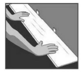
Begin installation working from left to right. Insert spacers at ends and edges where planks meet wall.
