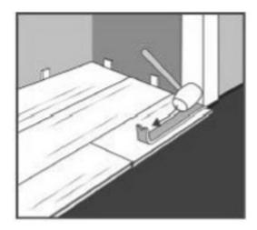
Use hammer and pull bar to lock short end of plank.
