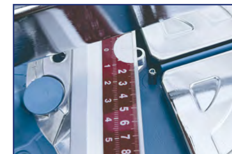
The measurement bar pivots on a steel pin at the centre of the cutting line, swiveling at +45° 0° - 45°.
